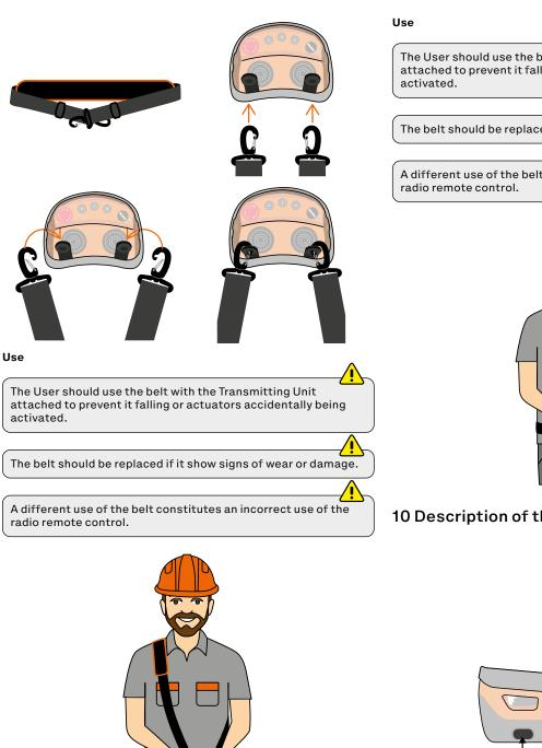
The User should use the belt with the Transmitting Unit attached to prevent it falling or actuators accidentally being activated.
