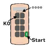
The white LEDs 1, 2 and 3 come on progressively depending on the charge status of the battery; if only LED 3 is on it indicates that the battery is low, LED 1, 2 and 3 on indicate that the battery is fully charged.
