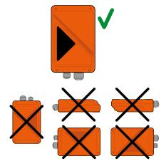
Fix the Receiving Unit in four points using the holes on the housing. Never put a hole in the Receiving Unit.
